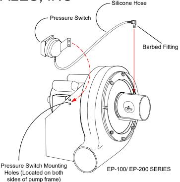
\*Connect the wire leads provided to terminals 1 and 2 labeled (C) Common and (NO) Normally Open.
