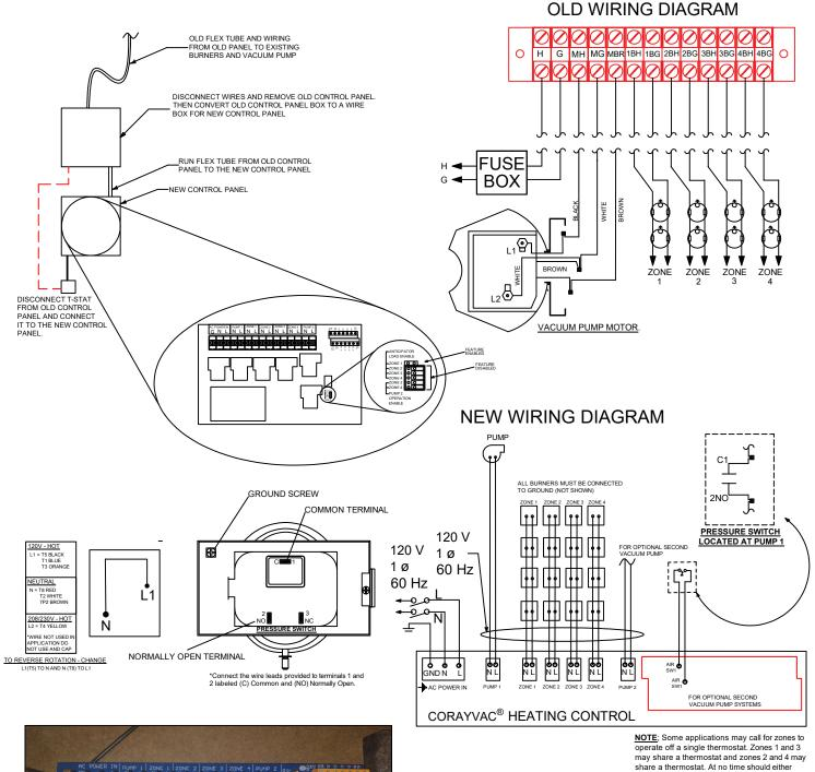
share a thermostat. At no time should either zone 1 or 3 be connected to zone 2 or 4. Doing so will result in damage to the control board.
